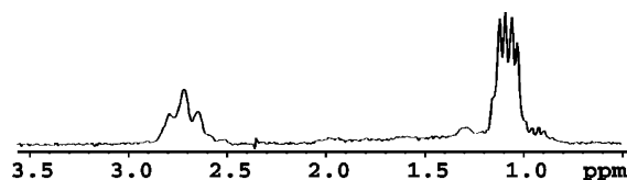
Figure 7. ^6\text{Li} NMR spectrum of the mixture of 0.13 M CH 3 C[ ^{15}\text{N} ], 0.26 M n -Bu[ ^6\text{Li} ], and 0.13 M [ ^{15}\text{N} ] 2 in Et 2 O- d 10 at -87\text{ }^\circ\text{C} .
